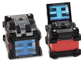
Supports bi-directional splicing operation
